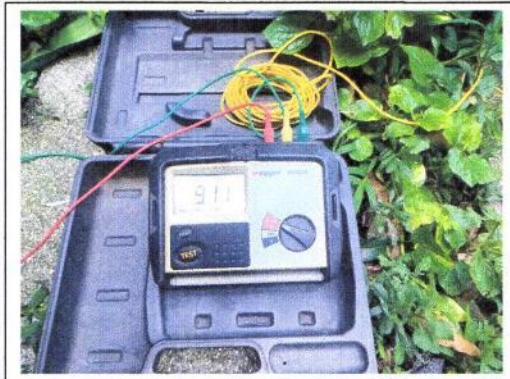
Picture 6: Capacitor Bank Check , Ground Resistance test .
